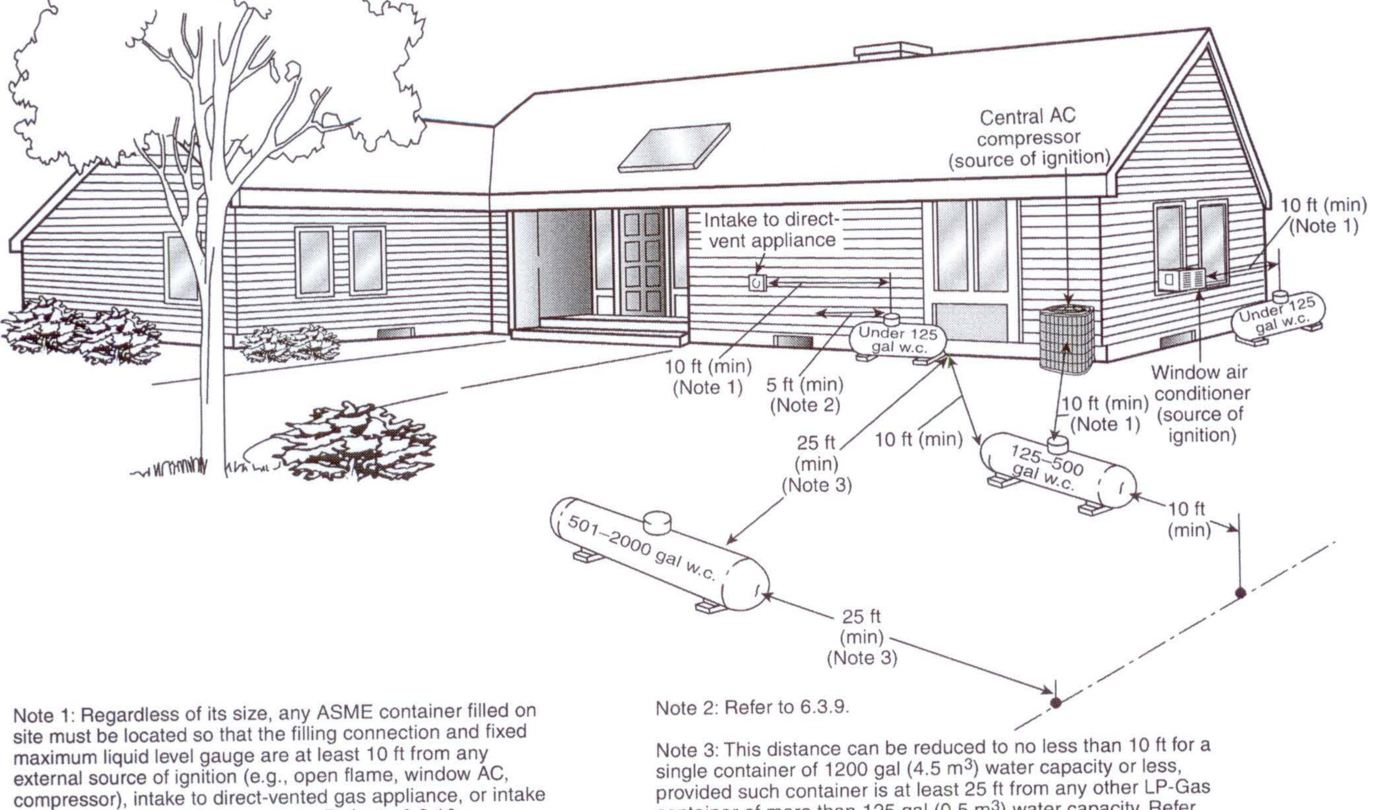
to a mechanical ventilation system. Refer to 6.3.10.
